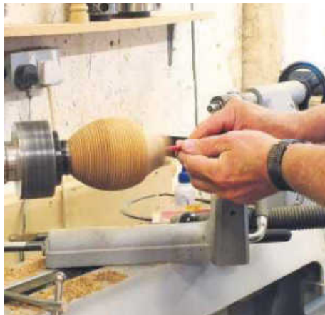
STEP 24. The important thing when sanding the inside of a piece like this is to not let go of the shaft. I also like to put the ball inside before I start the lathe and stop the machine before removing it
